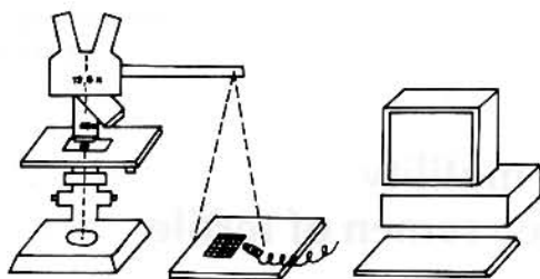
Figure 1 Diagram of the microscope equipped with a drawing tube, digitizing tablet with cursor, and microcomputer.
